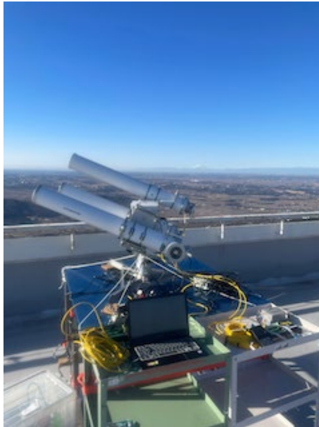
Photo 2. The collimation tube/pyranometer combination. A pyranometer was attached to the bottom end of the tube.
