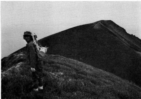
Photo. 6. The seismograph system which was used in the observation. The seismograph is essentially an ocean bottom seismograph (OBS), which has been slightly modified, contained in a waterproof plastic cylindrical case, for the land observation. The advantage of the land OBS is small and light, which weighs about 12 kg. It has a flat frequency response from 3 to 25 Hz. The recording period of the seismograph is 12 days.
