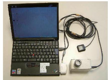
火山ガス観測装置：COMPUSS Compact Ultraviolet Spectrometer System
