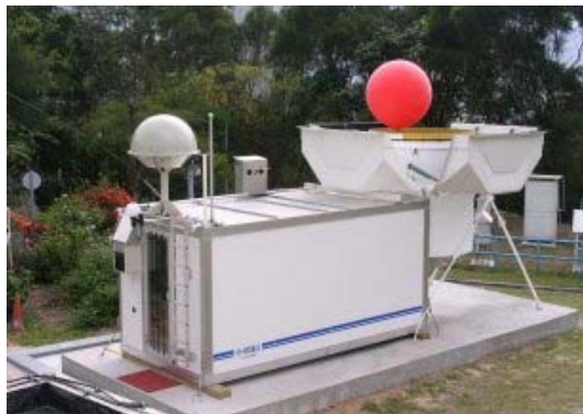
Automatic sounding station
