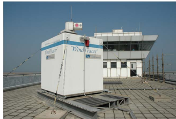
LIDAR for windshear detection
