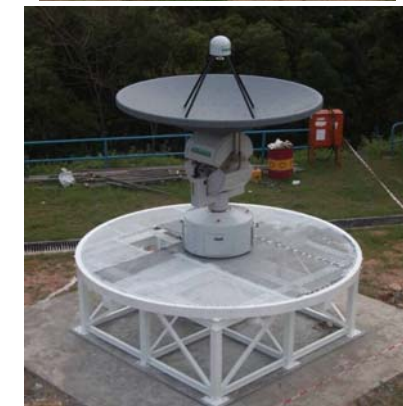
Tracking antenna for MODIS/POES at King's Park Meteorological Station
