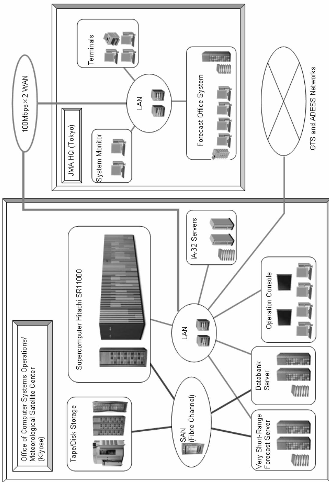
Figure 2.2.1 Schematic illustration of the computer system.
