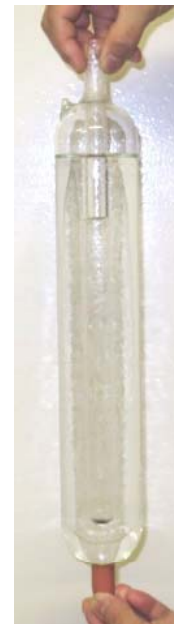
Water triple point cell
